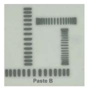
Both pastes were run through a reflow oven at 180°C. Paste B has better hot slump properties than Paste A and would less likely cause bridges, solder balls or mid-chip balling. For fine pitch components it is critical to select a lead-free paste with a heat stable gelling agent.
