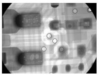
X-Ray, Voids in QFP joints
